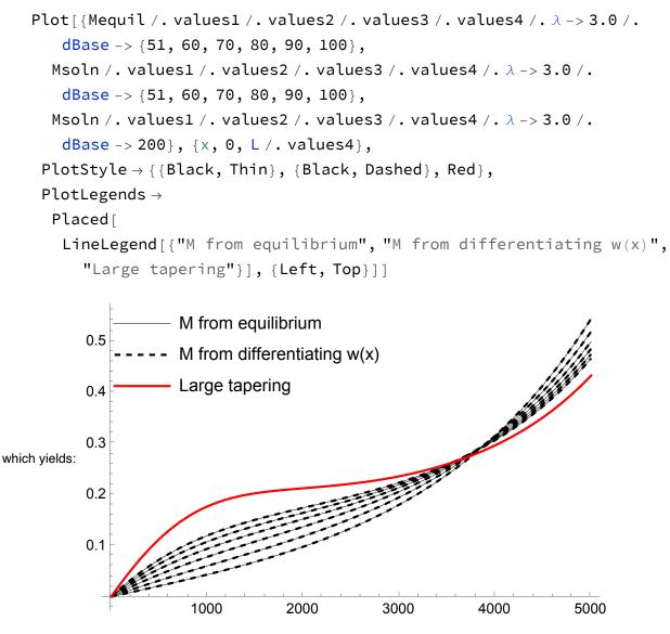
Also, keep in mind that the increasing stiffness at the base, from increased tapering, makes the cantilever overall stiffer. In turn, that may attract more lateral force, which could indeed make the moment at the base larger than without tapering.
