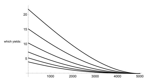
Bending moment diagram for different degrees of tapering, at constant force level; notice how the bending moment at the base diminishes with increasing cross-section diameter there, but the shape of the diagram changes:
