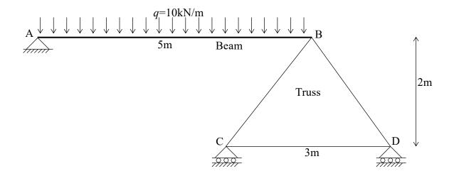
We start by determining the internal forces due to the externally applied real load, q, for this statically determinate structure by equilibrium:
