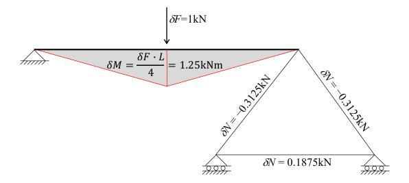
The sought displacement is now calculated by adding up virtual work, i.e., "virtual internal force times real internal deformation." Notice the use of quick-integration formulas for the integration of virtual moment with real curvature:
