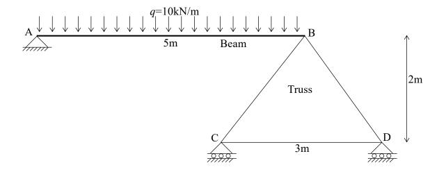
Because the structure is statically determinate, deformations do not affect the internal forces. That means the beam feels simply supported, regardless of the deflection at B. As a result, we start by analyzing the following simply supported beam:
