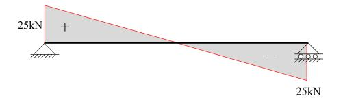
The shear force at B transfers to the truss structure below that point. Joint equilibrium at B starts with the transfer of the shear force in the beam onto the joint:
