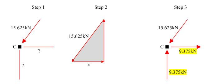
Similarity between the shaded triangle in the force polygon above and the shaded triangle below gives the axial force in the horizontal truss member:
