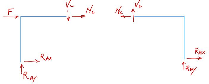
The figure above shows a total of six unknown forces. We can set up three equilibrium equations for each part of the structure, for a total of six equations. They are shown on the next page, for reference:
