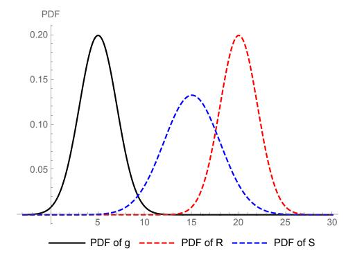
Calculating the failure probability by integration:
