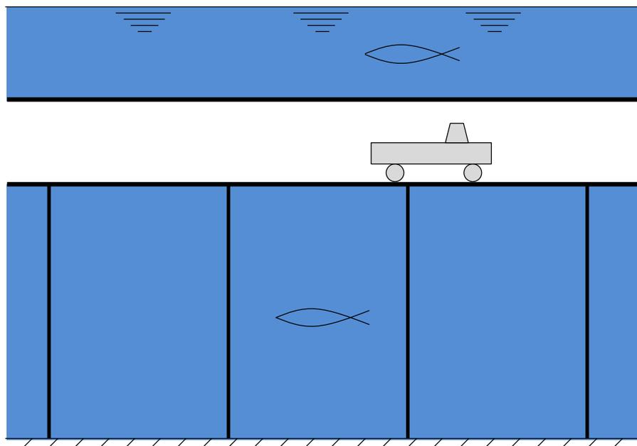
Figure 13: Submerged tunnel with tension legs.
