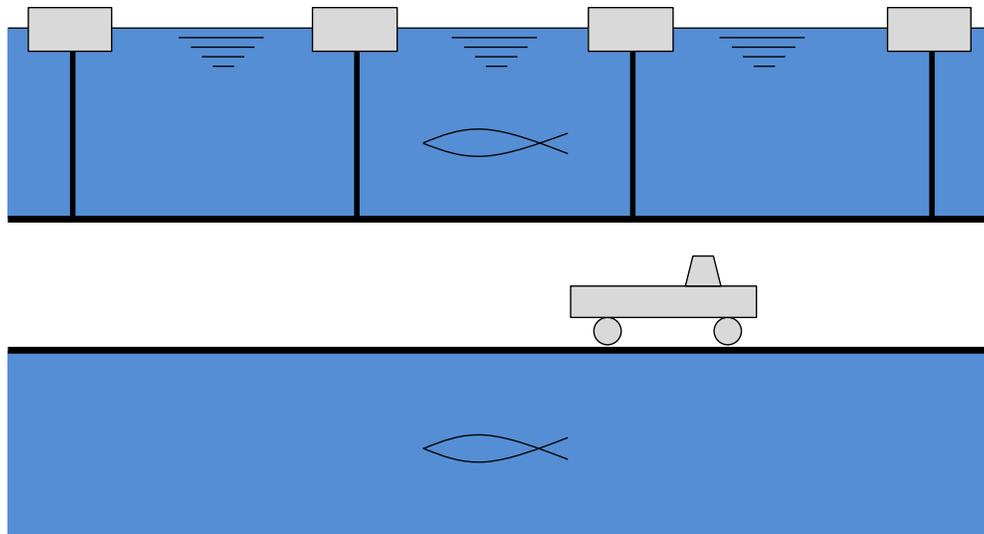
Figure 12: Submerged tunnel with pontoons.
