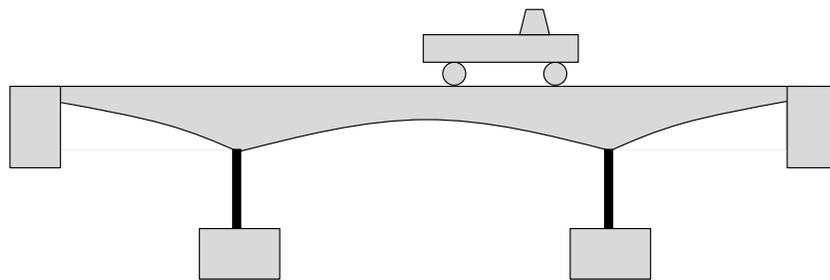
**Figure 10: Cantilever bridge.**
